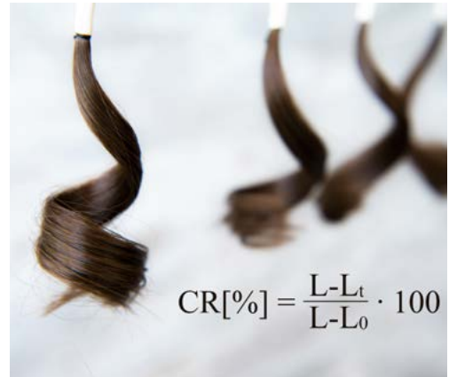
Fig. 1. Comparison change in length of curled hair swatches, 24 hrs. 80 % moisture.
